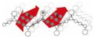
FIGURE 4: Dye is immobilized when bound to the aggregate and begins to fluoresce.
